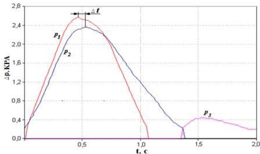
**Figure 2: Diagram of the Respiratory Cycle, Indicating the Time Displacement  $\Delta t$  between the Amplitudes of the Pressure Signals for Sensor P1 and P2, That Fixing the Air Flow Rate and Pressure Drop across the Nasal Cavity, Respectively, According to the Dynamic Data (AAR)**
