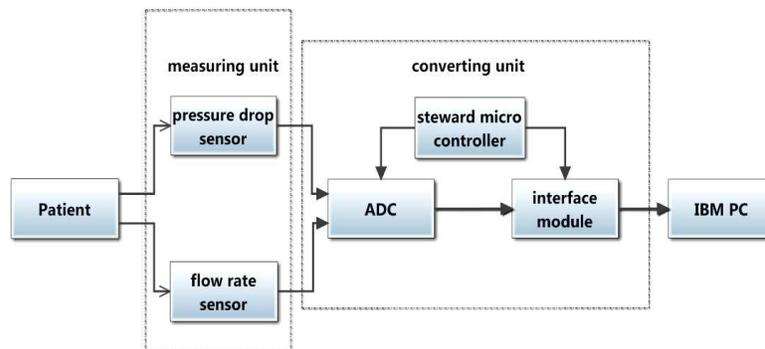
Figure 1: Schematic Diagram of the TNDA-PRH Device
